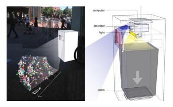
Figure 8: Architecture of Augmented Trashcan
